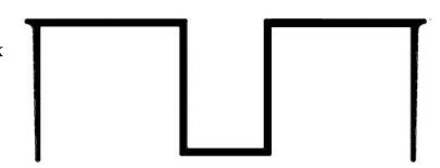
Model No. Wall Size SWCGT-212-2 2-1/2" stud w/ 1/2" GPDW for 3 1/2"Wall 2-1/2" stud w/ 5/8" GPDW for 3 3/4"Wall SWCGT-212-8
